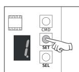
4 • The display will show the value 0 or 4. Use the SEL button to put on the desired option. Press the SET button once to save this option.
