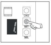
4 • The display will show the value 0 or 1, which identifies the option in which the control board is currently configured. Use the SEL button to put on the desired option. Press SET to save the option.
