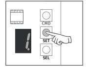
4 • The display will show the value 0 or 1, which identifies the option in which the control board is currently configured. Use the SEL button to put on the desired option. Press the SET button once to save this option.
