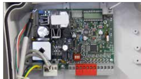
CT10224 control unit with integrated display
